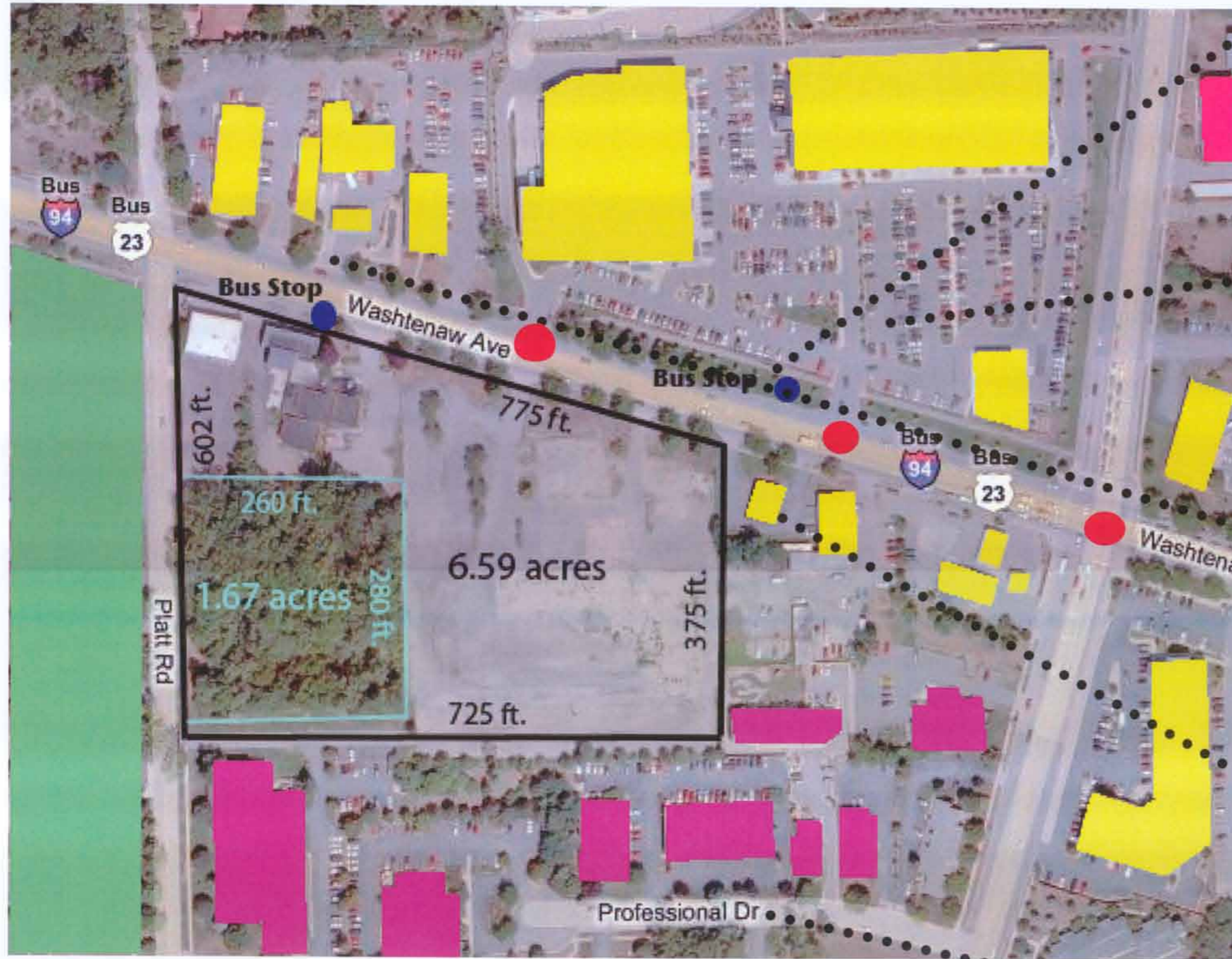
An AATA bus stop is located an at inconvenient distance from pedestrian crosswalk, causing pedestrians to cross traffic at 45 mph
